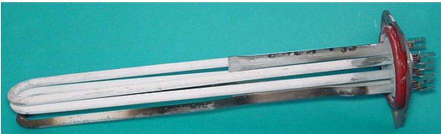
**Figure 2: Heating element with limescale deposits**
