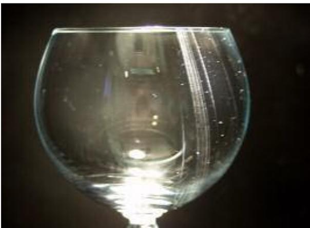
**Figure 3: Linear corrosion**
