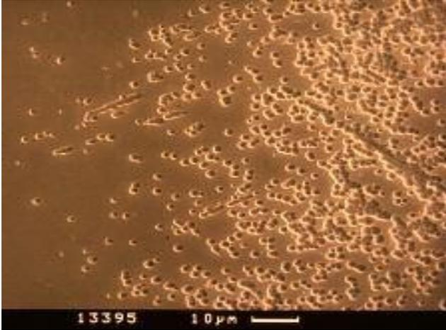
**Figure 2: microscopic view of the glass corrosion**
