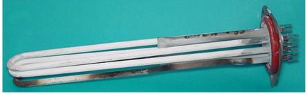
Figure 2: Heating element with limescale deposits Source: Miele & Cie. KG
