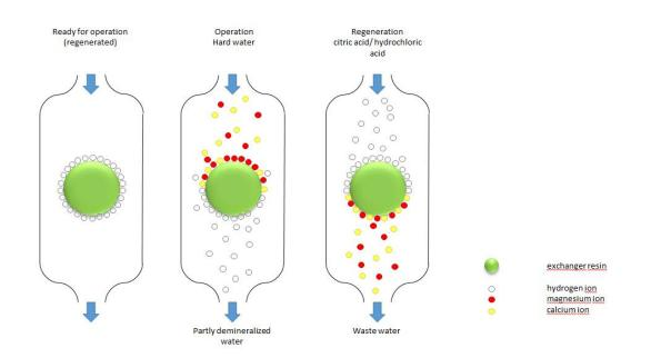
Figure 4: Partial water desalination Source: Miele & Cie. KG
