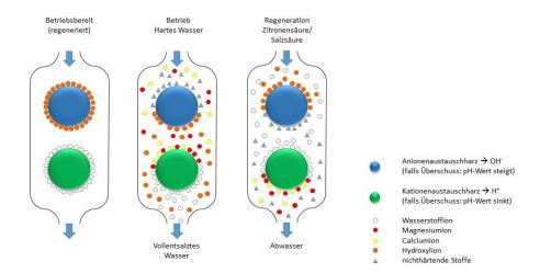
Figure 5: Full desalination through ion exchange Source: Miele & Cie. KG
