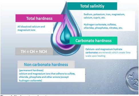
Figure 1: Hardness types in water Source: Brita Professional GmbH & Co. KG
