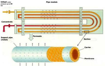
Figure 6: Structure of a reverse osmosis module Source: Ecolab
