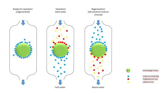
Figure 3: Water softening Source: Miele & Cie. KG
