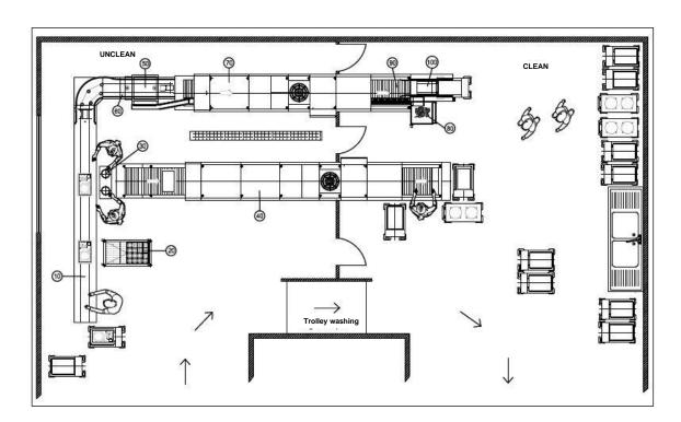
Figure 4: Planning example of a dishwashing system in a main hospital kitchen Source: Hobart
