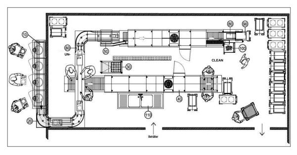
Figure 3: Planning example of dishwashing area in a canteen with flight-type dishwashers Source: Hobart
