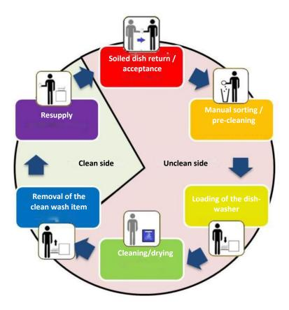
Figure 1: Functional areas in the wash item circuit
