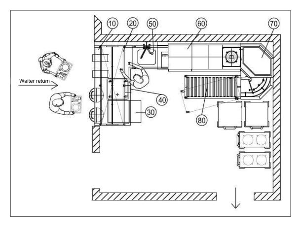
Figure 2: Planning example: Restaurant and banquet with rack conveyor dishwasher Source: Hobart
